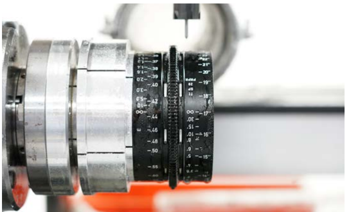
The order goes in to the engraving department, and an NP scale is made immediately. Notice that one focus ring has both feet and meters.
