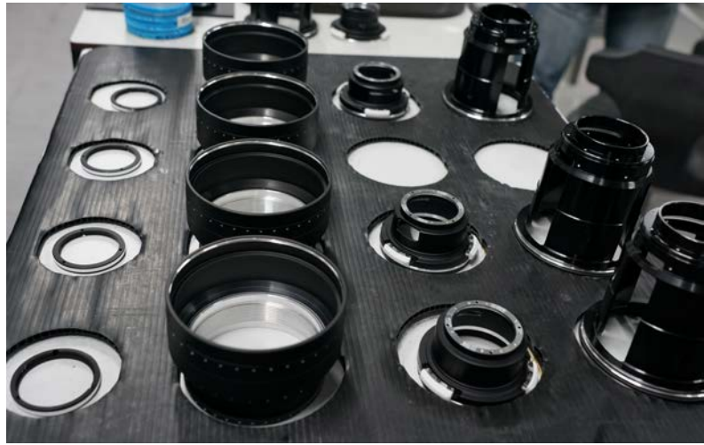
Inside the innovative focus mechanism: rectangular helical threads, precision CNC machining and advanced materials for smooth moves.
