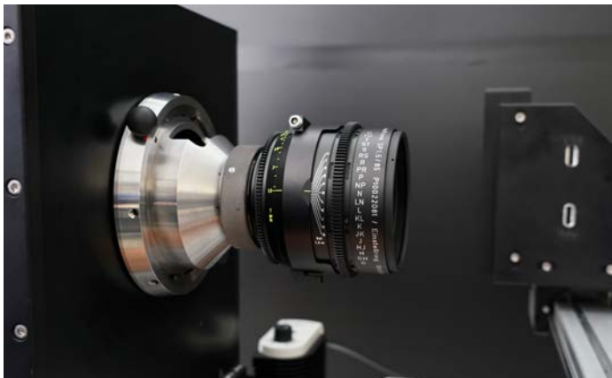
The lens is focused and the shows which scale is appropriate. In this example, the sharpest image is between N and P, so an NP scale is requested.
