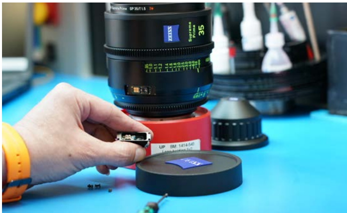
Connector removed, revealing electronics board beneath.
