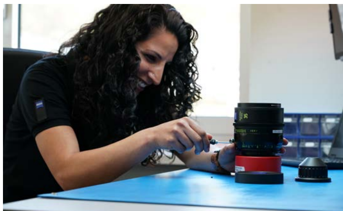
Servicing the Supreme Prime's eXtended Data connector.
