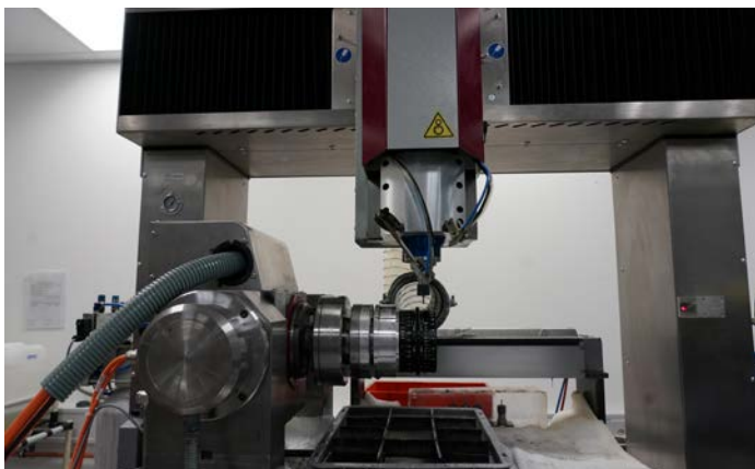
The order goes in to the engraving department, and an NP scale is made immediately. Notice that one focus ring has both feet and meters.
