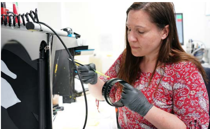
The lens is painted with steady hands, dried, and sent one floor up, back to the assembly department — to be fitted on the lens.
